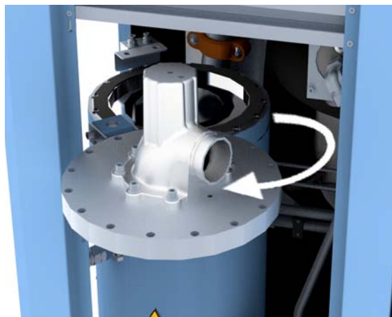
Fig. 6.19: Opening the lid of the compressed air-oil filter
