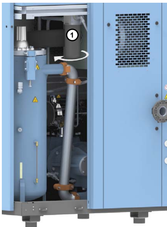
Fig. 6.10: Changing the oil filter
